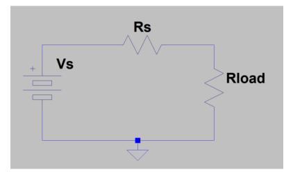
Note that this is a Thevenin Equivalent source with a load resistor.
