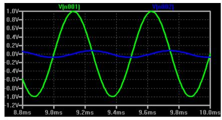
Simulated RC at 2 kHz
