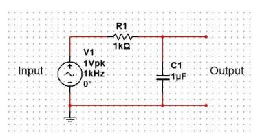
This circuit has a time constant  $t = RC = 10^{-3}$  which corresponds to a 3 dB point at  $1/(2pi*10^{-3})$  which is approximately 159 Hz where the voltage gain is 0.7071 and the phase shift is 45°. The gain of this circuit is always less than 1 and the Phase shift never exceeds 90°.
