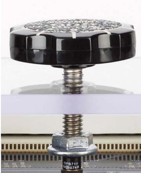
Figure 9.16: Optical position sensor (bottom) and target position knob (top) on QNET mechatronic sensors trainer.
