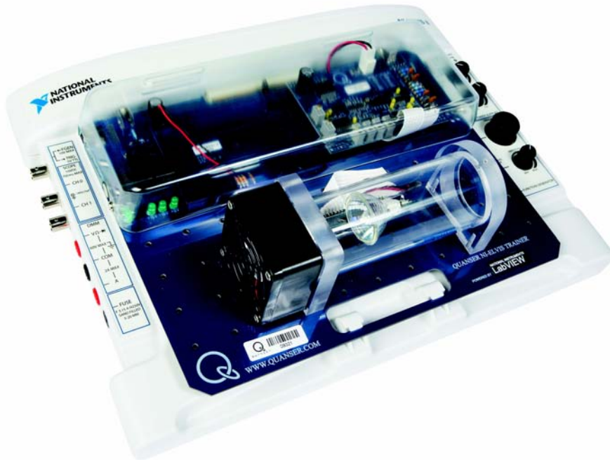
Figure 5.1: The QNET heating and ventilation trainer (HVACT).
