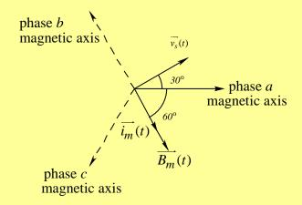
$$\overrightarrow{i_{ms}} = \frac{\overrightarrow{v}_s}{j\omega L_m} = \frac{254.56 \angle (30^0 - 90^0)}{2\pi \times 60 \times 0.777} = 0.869 \angle -60^0 A$$
